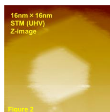
Figure 1 shows a molecular resolution STM image of triacontane self-organized on Cu (111) surface. Figure 2 shows a STM image of surfaces shown as figure 1 after heat treated in UHV.
